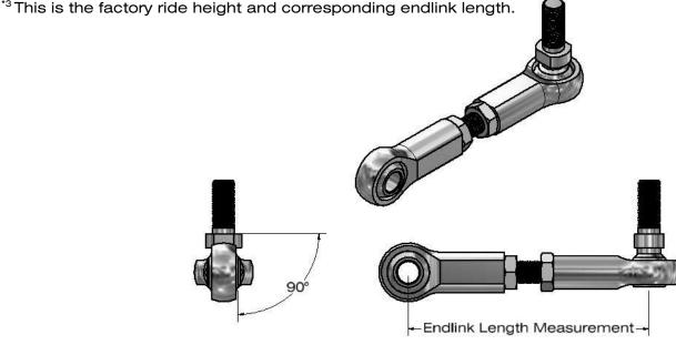
Assemble left and right endlinks with the provided female endlink halves, threaded rods, and 3/8" thin lock nuts. Build assemblies so the endlink halves are exactly 90 degrees in relation to each other. Make certain the lock nuts are tightened securely to the endlink halves by using two 9/16" open end wrenches.
