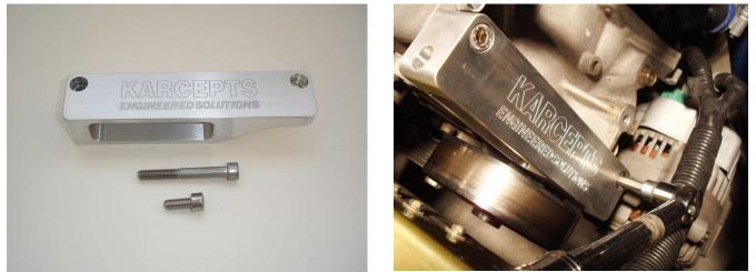
2. Insert the tensioner block into the tensioner bracket with the tapped hole in the tensioner block facing upwards. Temporarily snug the M8 x 25mm button head cap screws, lock washers, and flat washers into place with the tensioner block resting in the bottom of the tensioner bracket.
