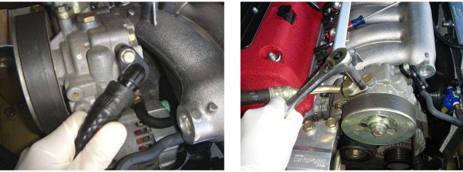
2. Relieve tension on the factory belt by rotating the bolt on the auto-tensioner pulley clockwise, and remove the belt.
