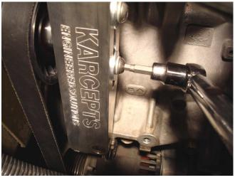
6. Once the tensioner block has been locked into place, the adjustment bolt will now be relieved of its tension. Because of this, you will want to tighten the adjustment bolt <sup>1</sup>/<sub>4</sub> turn (90 deg) more in order to secure it in place.
