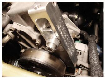
Insert the M8 x 60mm long socket head cap screw into the top of the tensioner bracket (leave loose temporarily; as shown).
