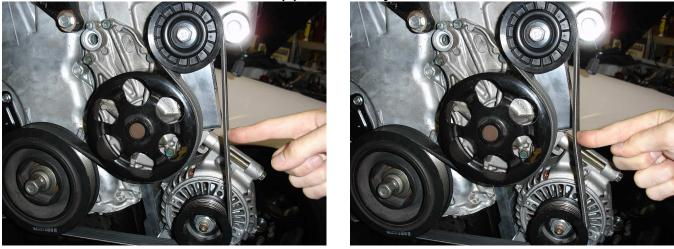
5. After belt tension is set appropriately, you may now torque down the button head socket cap screws. Torque both bolts to no more than 15 ft-lbs (180 in-lbs).
