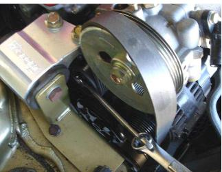
3. Unbolt the power steering pump and auto-tensioner from the engine.
