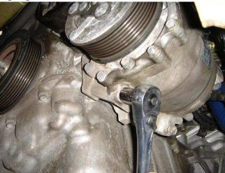
2. Unbolt the A/C compressor mounting bracket from the engine.
