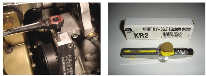
3. On a new belt, you want to set the initial static belt tension such that the Krikit II reads 140lbs. NOTE: This setting is higher than desired for normal operation, but is necessary for proper break-in. Run the engine for 3-5 minutes at this setting. After break-in is complete, re-tension to 100 lbs. Re-tension every 5,000 miles.
