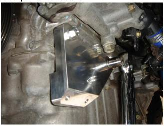
Locate the alternator spacer(s) (either 1 or 3 spacers are included, depending on Karcepts Kit Part # being used), the single M8 x 100mm long flange bolt (Honda Part #: 95701-08100-08), and two M8 x 50mm or M8 x 70mm long flange bolts (Honda Part #: 95701-08050-08 or 95701-08070-08). M8 x 70mm bolts are used when 3 spacers are provided.
