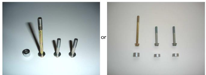
3. To prevent arcing, it is advised to first disconnect the negative and positive battery cables. Next, unbolt the alternator and discard the factory bolts.
