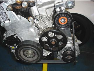
5. Install the bearing cover (Honda Part #: 31185-PCX-003) and M10 x 25mm special flange bolt (Honda Part #: 90031-PRA-000). Torque to 32 ft-lbs.
