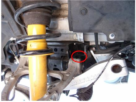
6. On the right side of the vehicle, remove the 2x M6 bolts holding the coolant pipe with a 10mm wrench and lower the plastic bracket out of the way.
