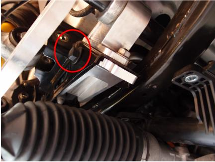
12. With the bolts loose, there may be a gap between the brace and the top sheet metal of the sway bar mounting surface as shown below.
