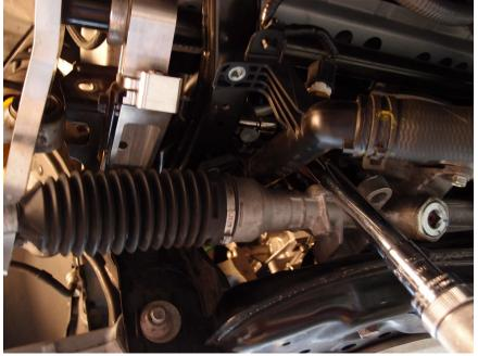
17. Re-install the M14 subframe nuts and torque to 100ft-lbs.
