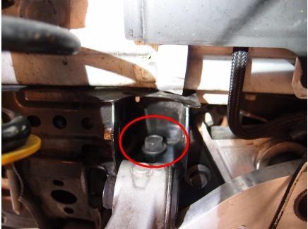
11. Thread in the side M12 x 20mm long bolts into the sides of the braces, near fully threaded, but still left loose.
