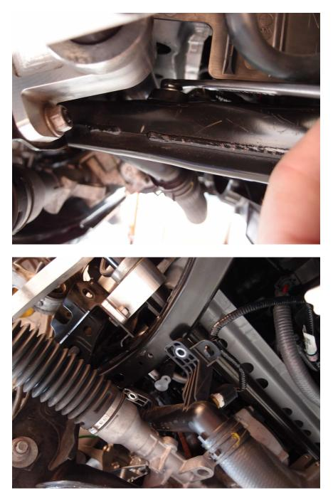
7. Put a few small drops of super glue onto one of the thick crush washers and glue 1x crush washer to the insides of the subframe as shown in the image below. Use the M10 bolt to guide and center the crush washer into place.
