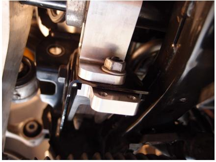
13. Push up on the bottom of the braces to close the gaps. While doing so, install the brace clamps with the M6 x 20mm socket head cap screws and tighten to EXACTLY 84in-lbs (7ft-lbs) of torque with a 5mm hex socket.
