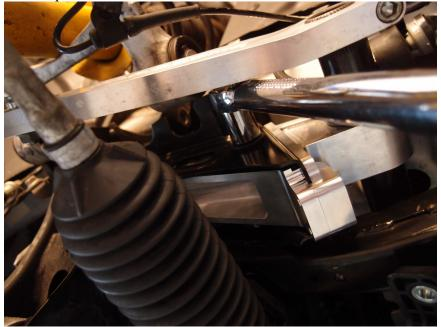
16. Torque the inside M10 bolt with an 8mm hex socket to 48ft-lbs.
