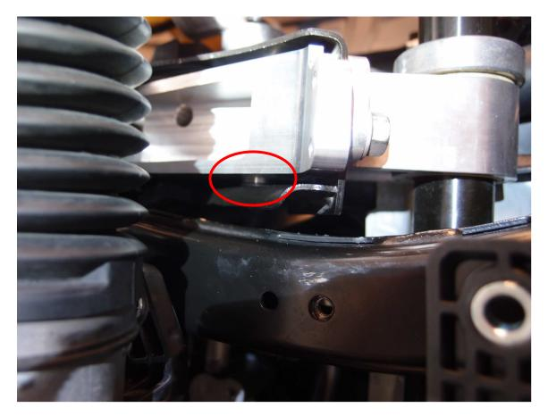
9. Install the remaining crush washers over the M10 x 25mm socket head bolts and install the bolts from the back side and thread into the braces. Screw in by hand almost to fully tight, but then crack loose to allow the brace to still flop around a little.
