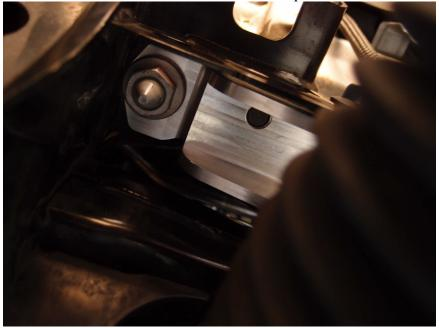
18. Brace installation is complete. Re-install the UCAs (45ft-lbs on the OE UCA bolts), ABS bracket, coolant pipe bracket, under tray, fender liners and wheels.
