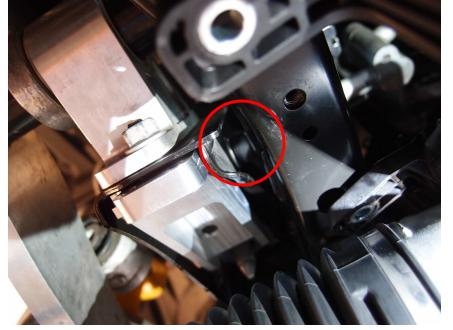
10. Thread the top M12 x 25mm long bolt by hand into the top of the braces. Screw in almost fully tight, but then leave loose, just like the M10 bolt.
