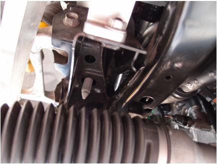
5. Remove the ABS sensor bracket from the UCA as well as the 2x bolts holding the UCA to the subframe and pull the UCA out of the subframe. No other bolts need removed. We are just looking for access to the top hole inside the front of the subframe. The damper body will hold the UCA from dropping too far,
