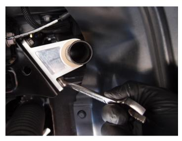
F. Slide the clamp collars over each end of the splined center section, push them tight against the mount bushings, and torque clamp collar set screws to 11 ft-lbs (132 in-lbs) with a 3/16" hex bit socket. Make certain there is no clearance between the bushings of the solid mounts and the collars once torqued.
