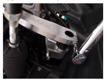
C. Rotate the sway bar arms upward until they make contact with the upper control arms. Compare the distance between the crossmember and the back of each sway bar arm as shown below. To verify the bar has been centered properly, an equal gap of approximately 1/4" will be observed on each side.
