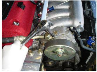
2. Relieve tension on the factory belt by rotating the bolt on the auto-tensioner pulley clockwise, and remove the belt.
