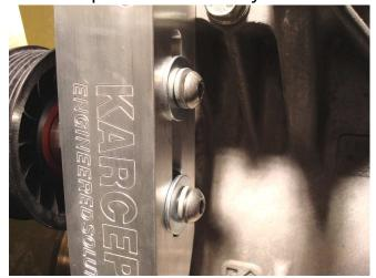
2. Tighten on the adjusting bolt to set proper tension. Tensioning may be performed with a Krikit II V-Belt Tension Gauge which can be ordered through any NAPA auto parts store. It's a very inexpensive yet handy tool!
