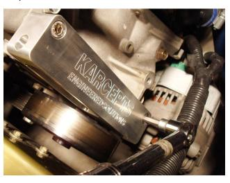
2. Insert the tensioner block into the tensioner bracket with the tapped hole in the tensioner block facing upwards. Temporarily snug the M8 x 25mm button head cap screws, lock washers, and flat washers into place with the tensioner block resting in the bottom of the tensioner bracket.
