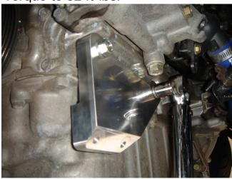
2. Locate the alternator spacer, the single M8 x 100mm long flange bolt (Honda Part #: 95701-08100-08), and the two M8 x 50mm long flange bolts (Honda Part #: 95701-08050-08).
