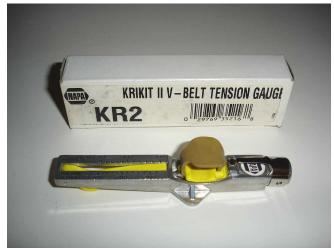
3. On a new belt, you want to set the initial static belt tension such that the Krikit II reads 140lbs. NOTE: This setting is higher than desired for normal operation, but is necessary for proper break-in. Run the engine for 3-5 minutes at this setting. After break-in is complete, re-tension to 100 lbs. Re-tension every 5,000 miles.
