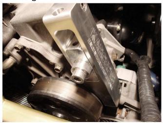
3. Insert the M8 x 45mm long socket head cap screw into the top of the tensioner bracket (leave loose temporarily; as shown).
