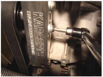
6. Once the tensioner block has been locked into place, the adjustment bolt will now be relieved of its tension. Because of this, you will want to tighten the adjustment bolt 1/4 turn (90 deg) more in order to secure it in place.
