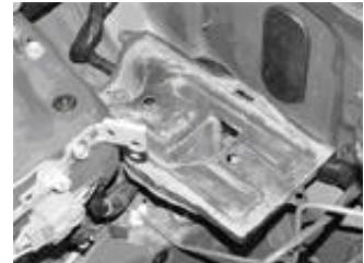
13. Install RSX shifter cables on the transmission. Route the shifter cables into the Civics' cabin by cutting a small hole in the floor in front of the old shifter location or low on the firewall. Check clearances with items like sway bars and catalytic converters to choose the best path. (Needle-Nose Pliers & Die Grinder with Cutoff Wheel)
