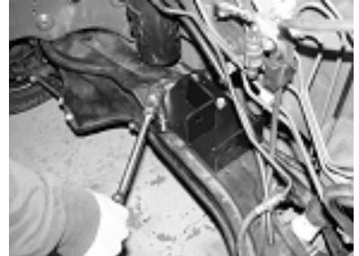
4. Place the new bracket on the framerail so that the elongated  $\frac{1}{2}$ " holes on the bottom of the bracket are centered over the lower transmission mount's boltholes, and the bracket is flush to the framerail. On top of the bracket there are two similar holes that are directly above the holes on the bottom of the bracket. Mark the center of these holes and then drill  $\frac{1}{2}$  inch holes into the top of the right-hand framerail.
