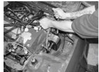
7. Place the rear mount in the rear bracket. Using the 12mm X 120mm bolt, 12mm locknut & 2-12mm flat washers, supplied in the rear-mount hardware bag, attach the mount to the bracket; do not tighten the lock nut yet. Next put the 12mm X 80mm bolt through the top bolthole and finger tighten a 12mm locking nut to it. (No Tools Required)
