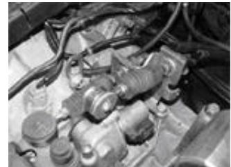
14. Install the left and right Hasport EGKAX axles, put the suspension back together and the wheels on the car. (14mm, 17mm, 19mm, 32mm Socket & 17mm Wrench)
