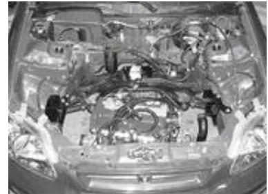
2. Place the left-hand bracket on the top of the transmission and insert the 12mm X 35mm bolts and washers, supplied in the left-mount hardware bag. A thick washer will be used under one of the holes on the rear of the bracket as a spacer. Snug the 12mm bolts down to the transmission but do not fully tighten them until all three mounts are in place. (17mm Socket)
