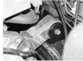
10. Torque all mount and bracket bolts according to specifications below. (14mm, 17mm, 19mm Socket & 17mm, 19mm Wrench)
